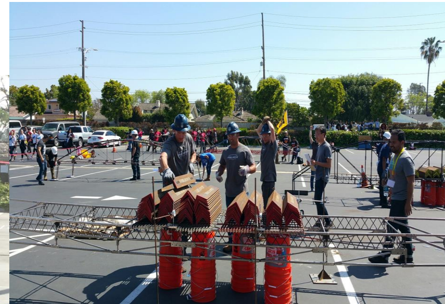
Figure 18: Vertical Load Test
